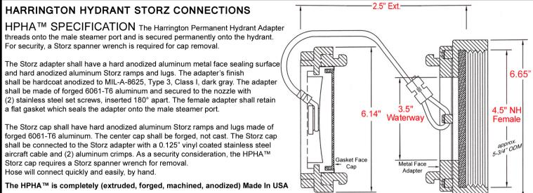
Once installed, the HPHA™ extends only 2.5" from the hydrant nozzle.
