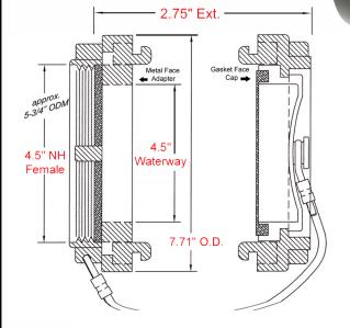
The Harrington Permanent Hydrant Adapter threads onto the male nozzle and is secured permanently to the hydrant. A Storz spanner wrench is required for cap removal.
