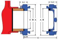
HPHA<sup>™</sup> only requires the removal of the threaded cap for installation
