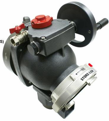
A low profile ball intake valve designed for pumper intake control. Valve meets 900 PSI hydrostatic strength test, utilizes full flow ball valve design and has easy-to-see visual indicator of ball position. Includes a 3/4" air bleeder valve, an integrated 25° elbow, and a 250 PSI Field adjustable pressure relief valve (adjustable from 75-250 PSI). The handle can be mounted on right or left side of valve.
