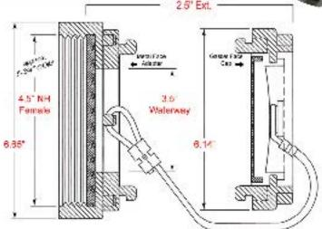
The Harrington Permanent Hydrant Adapter threads onto the male nezzle. and is secured permanently to the hydrant. A Sterz spanner wrench is requiree for eap removal.
