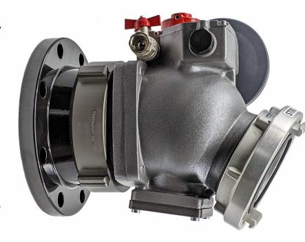
A low profile discharge ball valve designed for high flow applications. Valve meets 900 PSI hydrostatic strength test, utilizes full flow ball valve design and has easy-to-see visual indicator of ball position. Includes a 3/4" air bleeder valve and an integrated 25° elbow. The handle can be mounted on the right or left side of valve.
