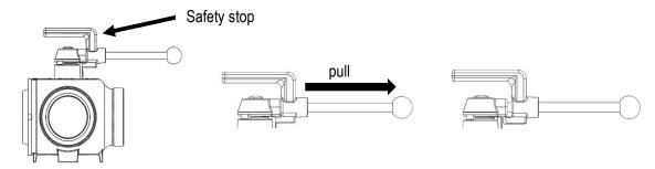
■ To change the water way from port A→B to A→C and D→B, turn the hand lever into the direction of the desired port. The safety device must be released before.
